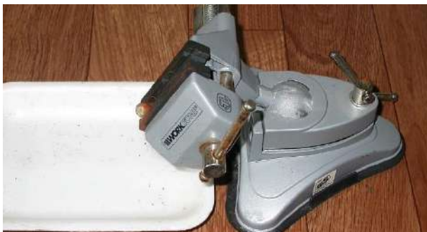
figure 3: Table-top vice suitable for controlled breaking of shells without crushing the soft parts.
